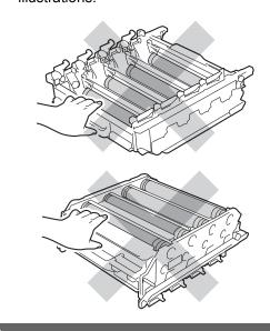
Turn the drum unit over by holding the green handles. Make sure that the drum unit gears (1) are on the left hand side.
